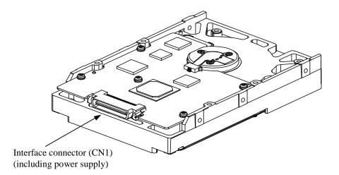
Figure 4.9 Connector location
