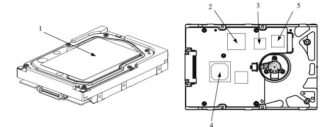
Figure 4.5 Surface temperature measurement points
