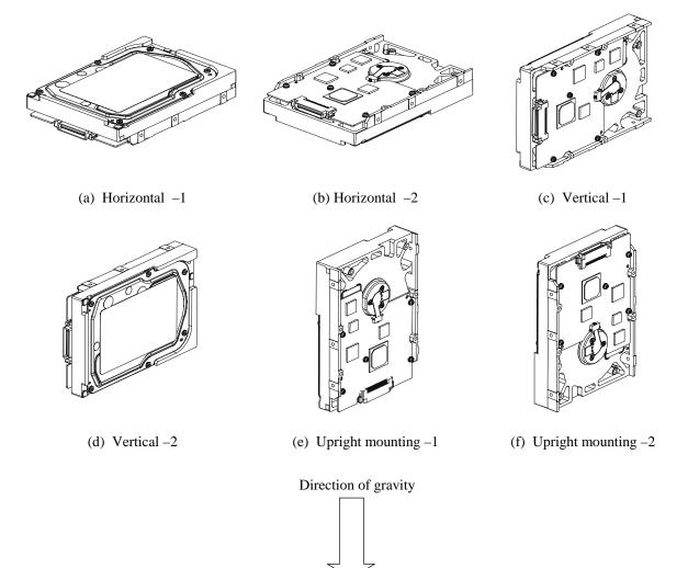
Figure 4.2 HDD orientations
