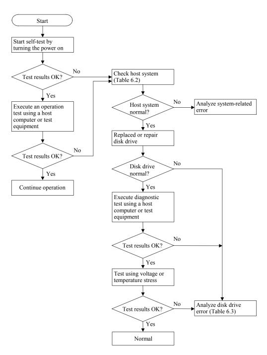
Figure 6.3 Test flowchart
