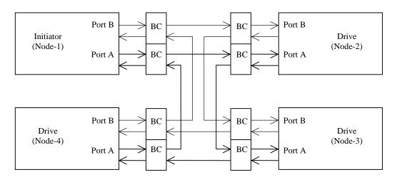
Figure 1.2 Example of FC-AL system configuration
