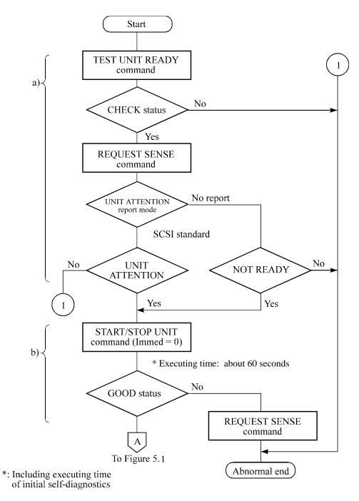
Figure 5.2 Checking the HDD connection (B)
