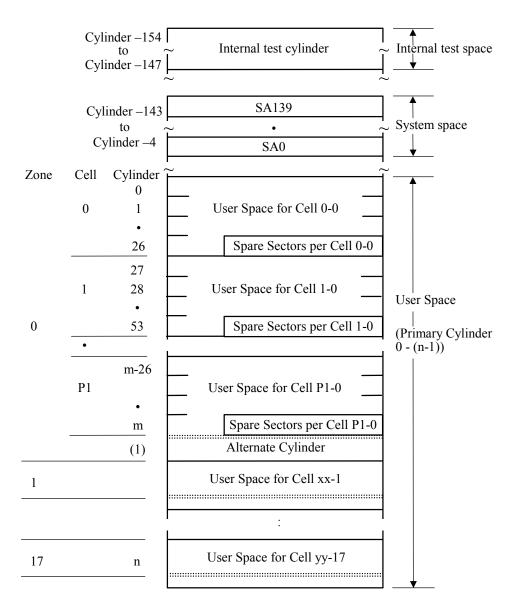
Note: Spare sectors on the last track in each cylinder are not necessarily placed at the end of the track because of a track skew or a cylinder skew. (Details are explained in Subsection 3.1.3.)
