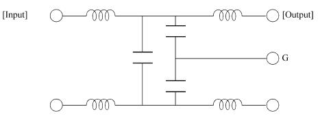
Figure 4.8 AC noise filter (recommended)
