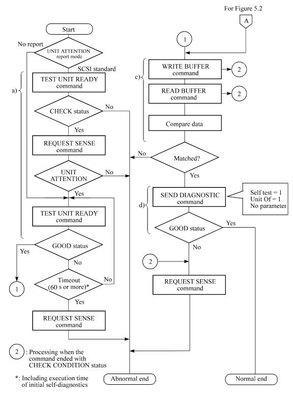
Figure 5.1 Checking the HDD connection (A)
