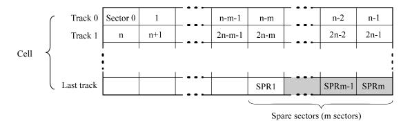
Note: This drive manages alternate spare areas for each cell, which is a set of cylinders. One cell consists of 27 cylinders.
