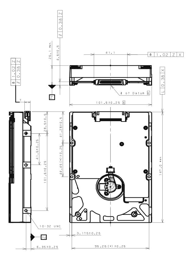
The value marked with (\*) indicates the dimension between mounting holes on the bottom face. [Unit: mm]
